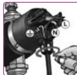
Fig 5. Electrical connection 1 x 230 V AC, 50 Hz, 0.11 A.
